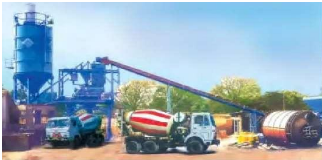
Modern ready mixed concrete plant.
