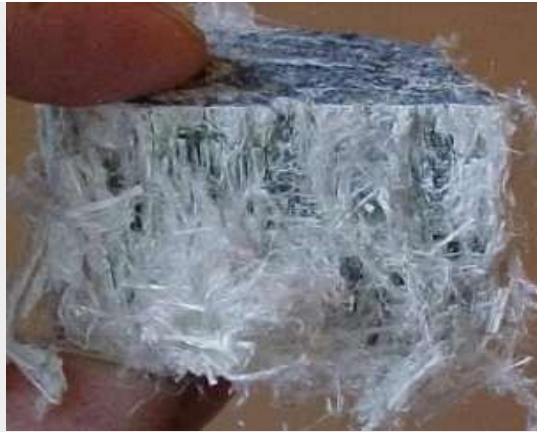
FIG-13 Asbestos fibers
